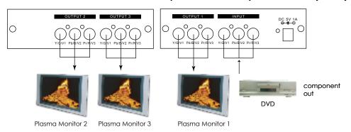
2. Works as a 1-in 3-out distribution amplifier for HD RGsB (Sync on Green) video source.
